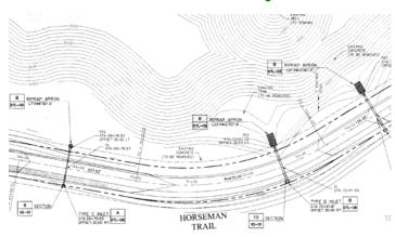
Frequently diverting stormwater flows from the cut side of the roadway to the fill side of the roadway, for a road designed with roadside ditches, is a great way to reduce the amount of stormwater carried in the cut side roadside ditch. Douglas County criteria has maximum depths for ditch conveyance for the minor and major storm design, which relates more to the impact the stormwater flows have on the roads ability to carry
