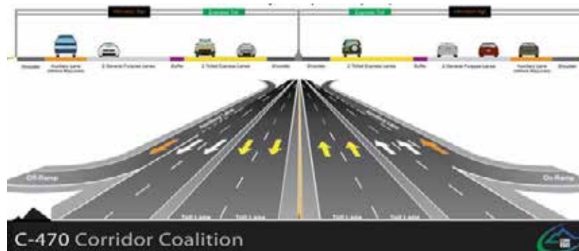
Ultimate Lane Configuration for C-470 is shown above for Full Buildout Section (providing for 2 managed toll lanes in each direction that are located in the center of C-470)
