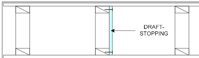
**FIGURE 10: Draftstopping at Open Web Trusses**
