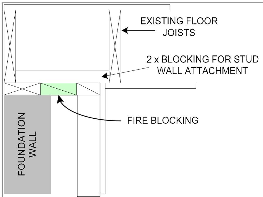
**FIGURE 6: Fire Blocking at Offset Stud Wall**
