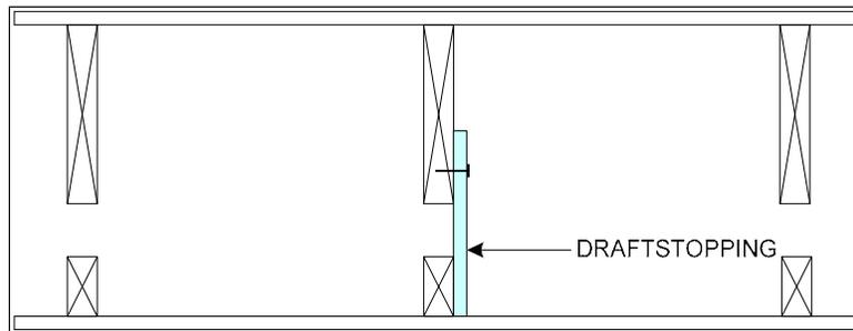
**FIGURE 9: Draftstopping at Drop Ceiling**
