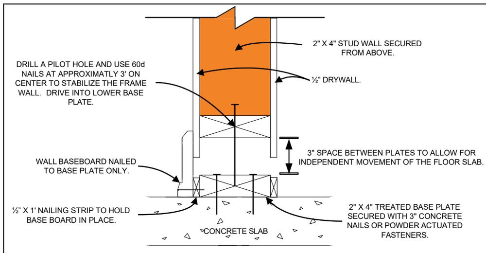
**FIGURE 8: Non-bearing Slab on Grade Wall Framing**
