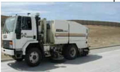
A vacuum or brush-type street sweeper is recommended to clean up any tracking of mud.
