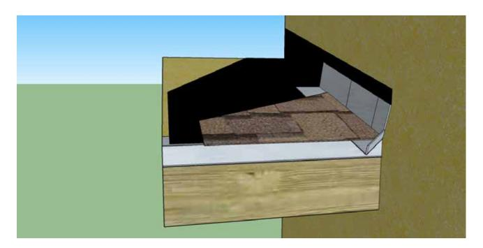
**IRC Section R905.2.8.3 Sidewall Flashing** – Base flashing against a vertical sidewall shall be continuous or step flashing and shall be a minimum of 4" in height and 4" in width and shall direct water away from the vertical sidewall onto the roof and/or into the gutter. Where siding is provided on the vertical sidewall the vertical leg of the flashing shall be continuous under the siding.
