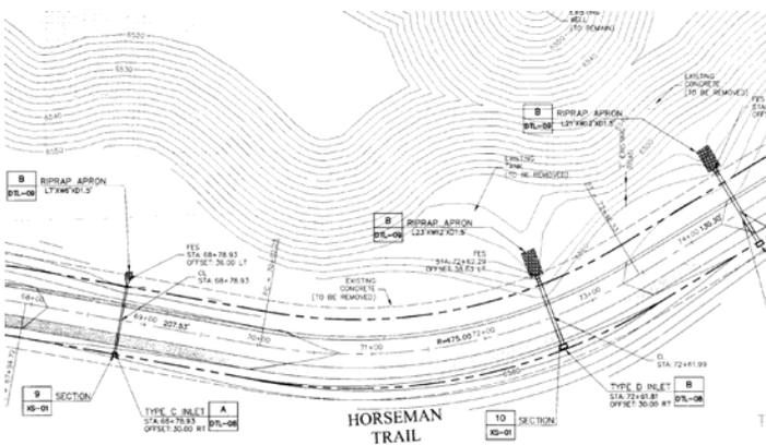
Frequently diverting stormwater flows from the cut side of the roadway to the fill side of the roadway, for a road designed with roadside ditches, is a great way to reduce the amount of stormwater carried in the cut side roadside ditch. Douglas County criteria has maximum depths for ditch conveyance for the minor and major storm design, which relates more to the impact the stormwater flows have on the roads ability to carry
