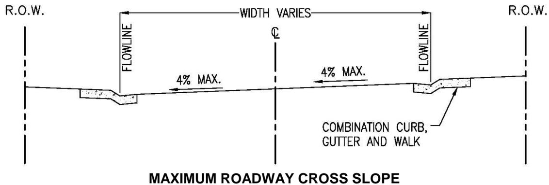
**The rate of change for roadway cross slope, when warping side streets at intersections, shall not exceed the following criteria:**
