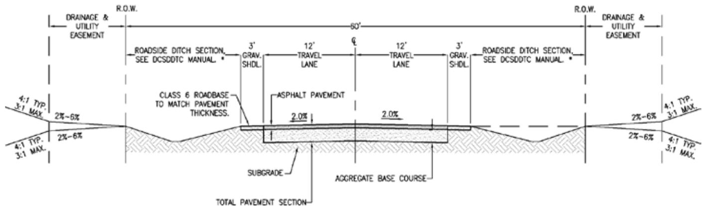
\* ROADSIDE DITCH MAY NOT BE REQUIRED IF THERE ARE NO CUT SLOPES ALONG THE ROADWAY.
