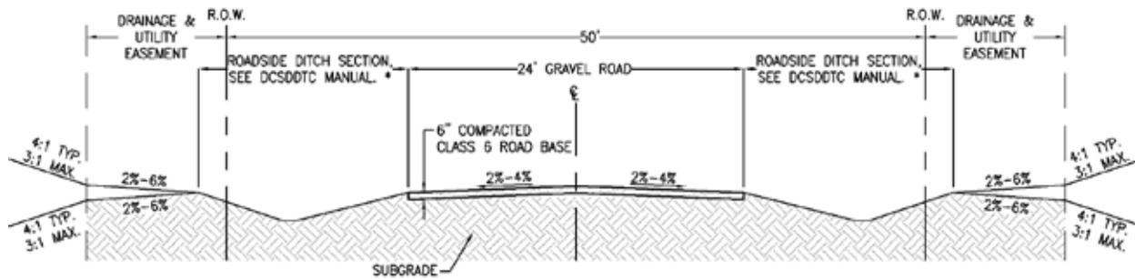
\* ROADSIDE DITCH MAY NOT BE REQUIRED IF THERE ARE NO CUT SLOPES ALONG THE ROADWAY.
