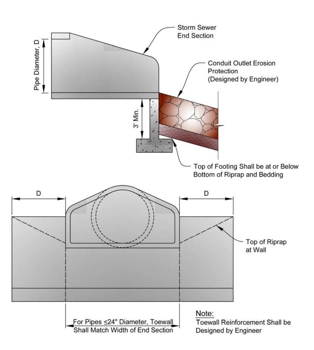
FIGURE 10-1 CONCEPTUAL TOEWALL DETAIL
